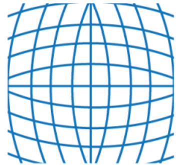
positive radial distortion "barrel"
